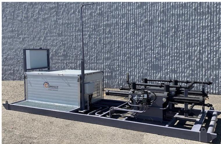
The increasing need for compression is accompanied by the need for higher flow rates and high differential pressure. Our multi-compressor systems incorporate 2 or more compression cylinders with a single small-footprint power pack to respond exactly to the required operating conditions.
