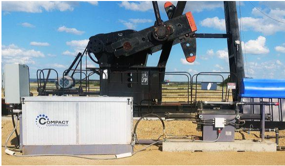
CCI HCG50 compressor operating in a casing gas compression application in Western Canada
