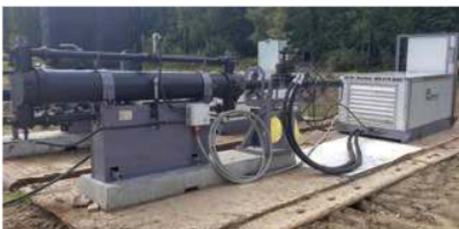
Fig. 1—Compact Compression's Multiphase Transfer Pump costs less than installing individual casing gas compressors on each well and has a lower service cost than previously available compressors in multiphase service.
