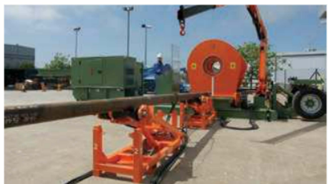
Fig. 2—EnerQuip's mobile torque machine provides a versatile drop-and-go platform for makeup and breakout services.
